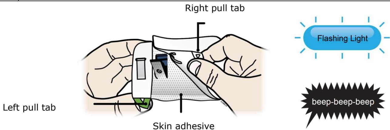
You must remove **both** green pull tabs to turn the loaded on-body infusor on. You will hear beeping and see a flashing blue status light.
