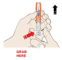
Once extended, the orange safety guard will lock into position and will not slide back over the needle.
