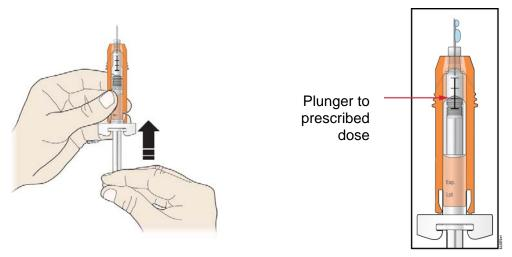
**Important: Do not** slide the orange safety guard over the needle before you give the injection. This will "activate" or lock the orange safety guard.
